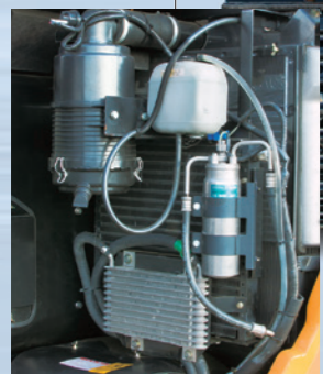
▲ Parallel configuration oil cooler and radiator make maintenance easier.
