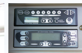
▲ FM/AM radio / switch panel for air conditioner
