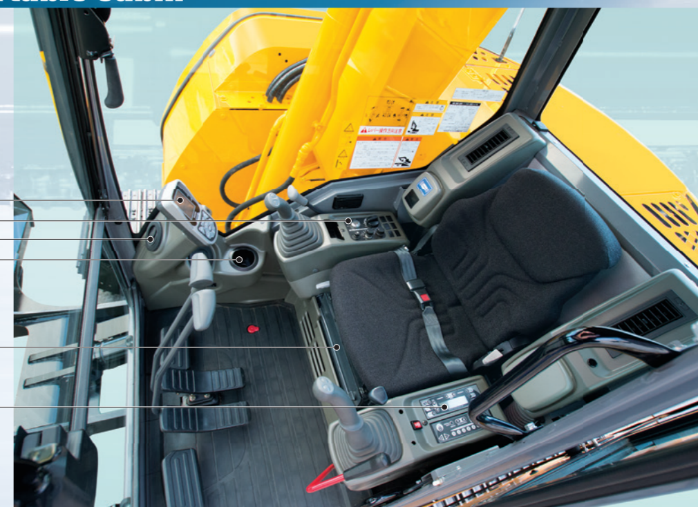
▲ The hour meter can be checked even when key is turned off.
